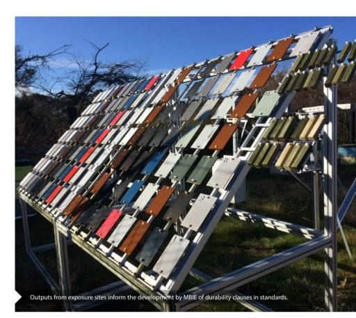
exposure to solar radiation) and left to react to nature at their own speed. Zhengwei visits each site at least once a year to observe and measure rates of corrosion and degradation in the samples.
