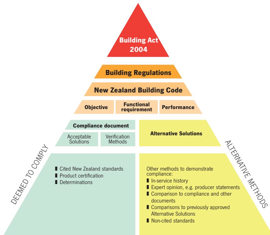
Hierarchy of New Zealand building controls. (Adapted from Department of Building and Housing drawing.)
