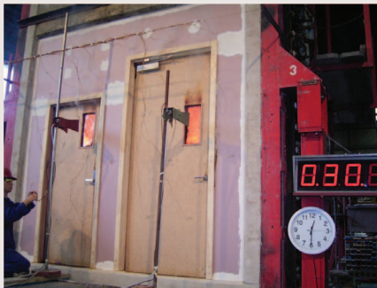
Figure 1: Fire door during testing at BRANZ.
